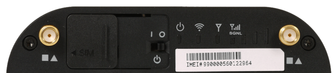
SIM SLOT/ON-OFF / LEDs / SIGNAL STRENGTH COR IBR600
